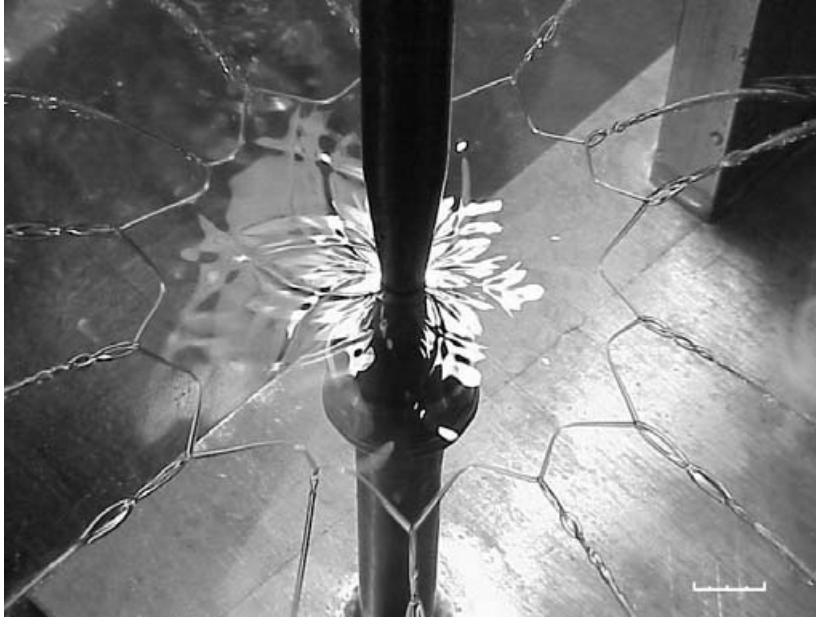
FIGURE 3. A polygonal fluid sheet (Buckingham & Bush 2001) generated by extruding a glycerine–water solution of viscosity 10 cS from a circular annulus of diameter 1 cm. Fluid chains are seen to emerge from the corners of the polygon. Scale bar: 1 cm.
